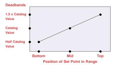
Temperature switch deadbands are a result of the characteristics of the vapor pressure curve as well as other factors. Normally, this results in a deadband which is narrower in the top third of the range than in the bottom third of the range. The values published are nominal and representative of midrange set points.
