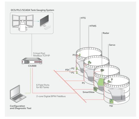
Figure 1: Architectural overview of a tank gauging system
