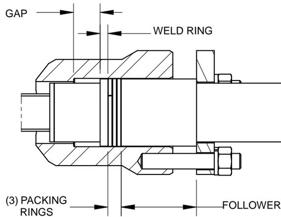
Figure 2-17 shows a view of the Pak-lok Annubar when installation is completed. Please note that there should be a gap between the Pak-lok Body and the Weld Ring.
