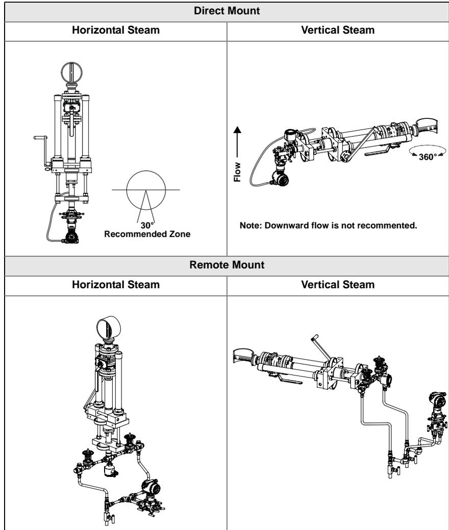
Figure 2-12. Top Mounting for Steam
