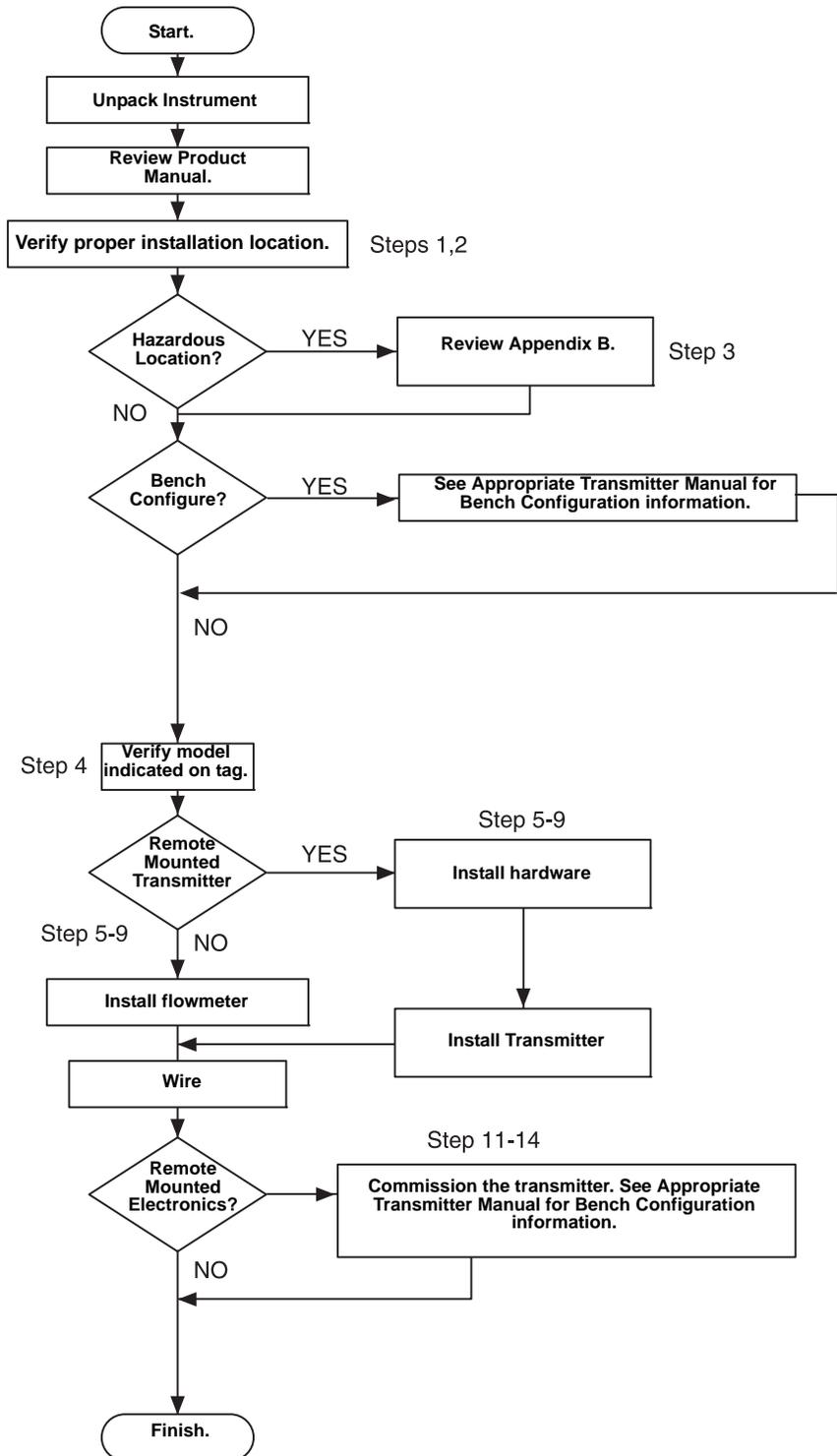
The following list is a summary of the steps required to complete a flowmeter installation. If this is a new installation, begin with step 1. If the mounting is already in place, verify that the hole size and the fittings match the recommended specifications (see Table 2-3 on page 2-19) and begin with step 5.
