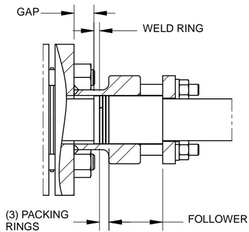
Figure 2-25 shows a view of the Flange-lok Annubar when installation is completed. Please note that there should be a gap between the Flange-lok Body and the Weld Ring.
