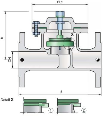
Tank connection for pressure relief function
