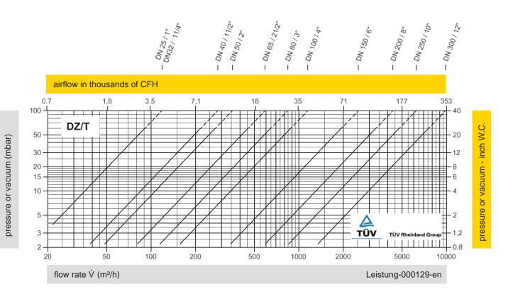
The flow capacity charts have been determined with a calibrated and TÜV certified flow capacity test rig. Volume flow  $\dot{V}$  in (m<sup>3</sup>/h) and CFH refer to the standard reference conditions of air ISO 6358 (20°C, 1bar). Conversion to other densities and temperatures refer to Vol. 1: "Technical Fundamentals".
