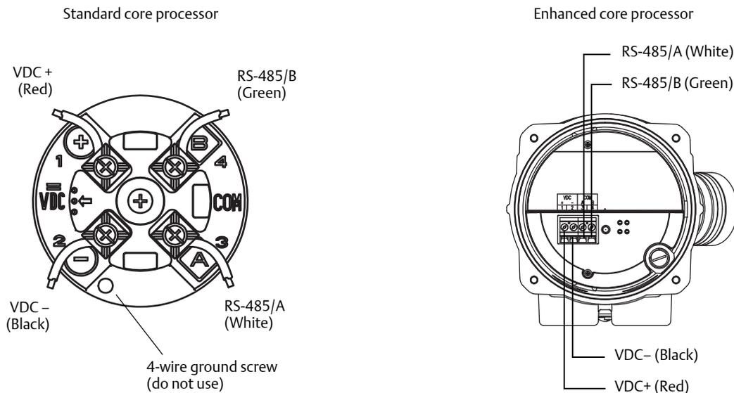
8. Connect power supply wires to the VDC terminals on the core processor (see [Figure 3-10](#)). If you are using Micro Motion 4-wire cable, use the red and black wires.
