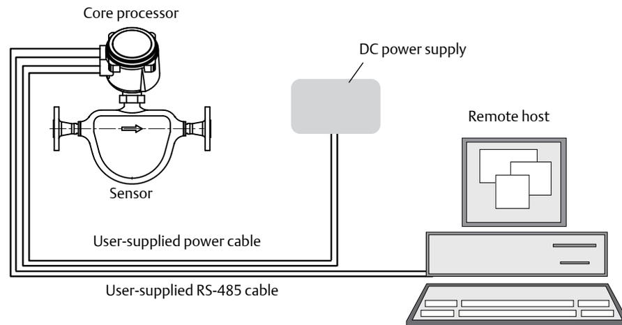
**Figure 2-2 MVD Direct Connect installations – Remote core processor, no I.S. barrier**
