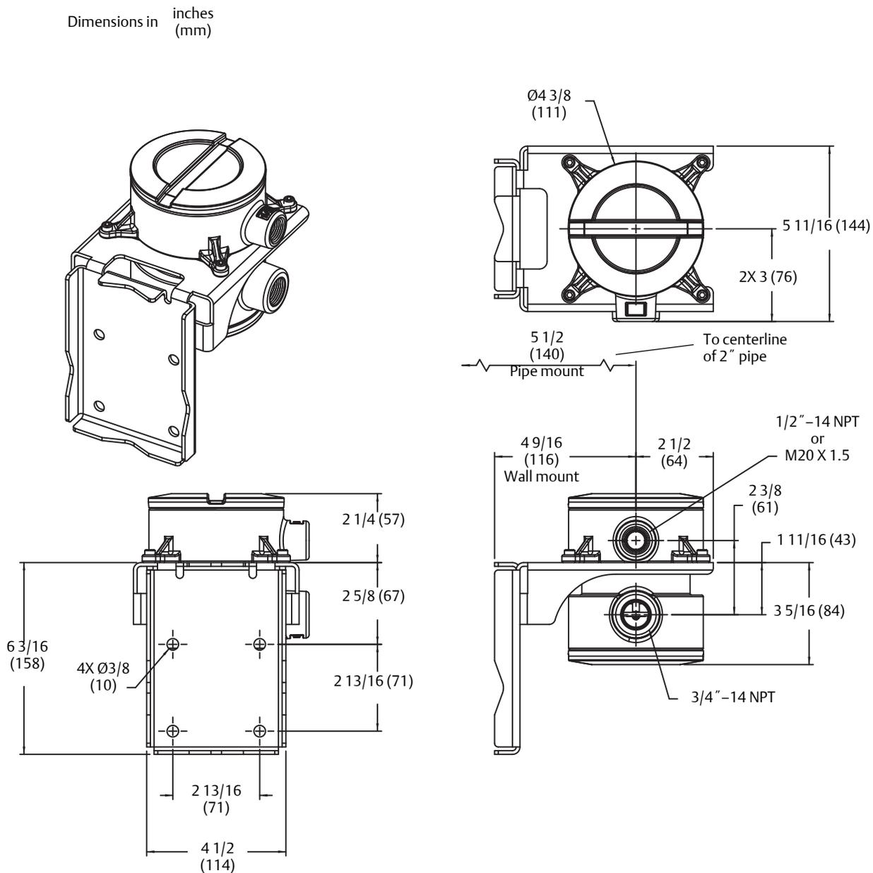
**Figure 3-4 Dimensions – Remote enhanced core processor**
