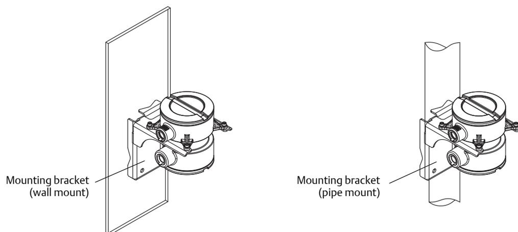
To mount the core processor:
