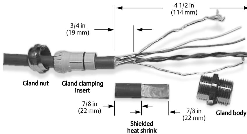
5. For connection at the core processor housing, prepare cable as follows (for armored cable, omit Steps 5d through 5g):
