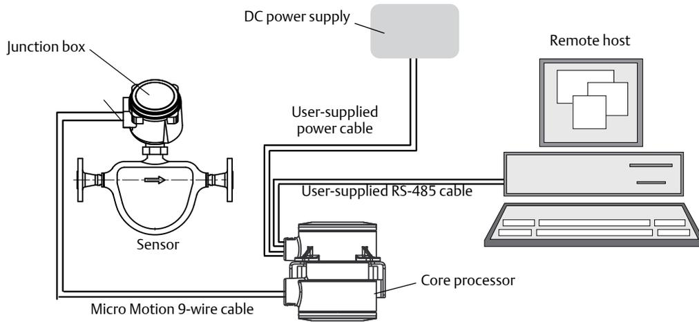
**Figure 2-3 MVD Direct Connect installations – Integral core processor, I.S. barrier**
