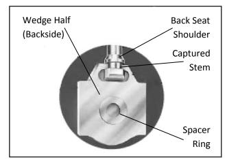
thousandths into the gate cavity, a 0.060 defect in one wedge seat drops the wedge more than three-tenths of an inch. The spacer ring provides a novel and inexpensive means of varying the wedge thickness either during manufacture or for field repair. A spacer ring of appropriate thickness can be installed for optimum wedge fitting, within the limits of the clearance in the wedge guiding system.
