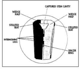
Figure 3 – Cutaway of Equiwedge Two-Piece Wedge
