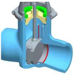
**Cutaway of Equiwedge Gate Valve**
