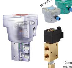
The balanced poppet design provides a uniform pressure field around the poppet that prevents any resistance to pressure when the valve opens. The coil therefore only has to offset the friction of the seal.
