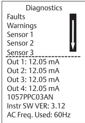
Information about each condition is quickly accessible by pressing **DIAG** on the keypad. User help screens are displayed for most fault and warning conditions to assist in troubleshooting.
