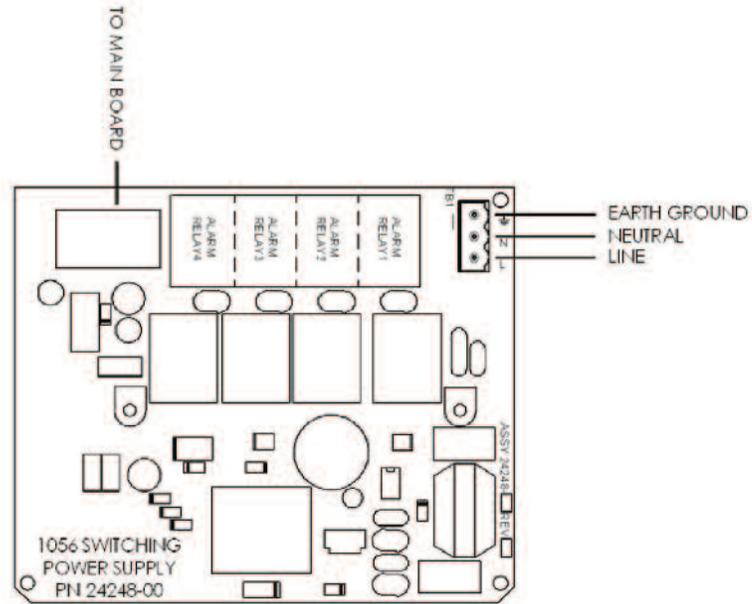
Figure 3-8 Output Wiring for Model 1057 Main PCB
