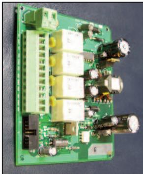
This power supply automatically detects DC power and accepts 20 Vdc to 30 Vdc inputs. Four programmable alarm relays are included.
