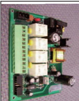
This power supply automatically detects AC line conditions and switches to the proper line voltage and line frequency. Four programmable alarm relays are included.
