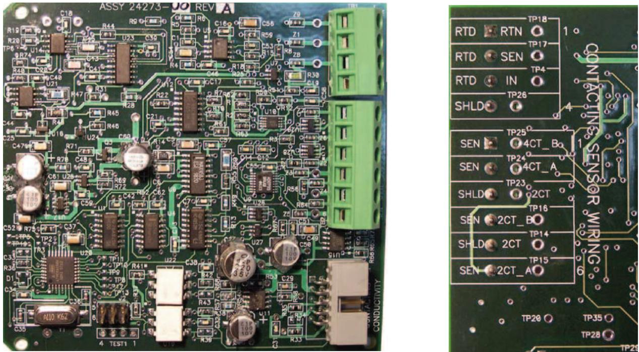
Figure 3-6 pH/ORP/ISE Signal Board and Sensor Cable Leads
