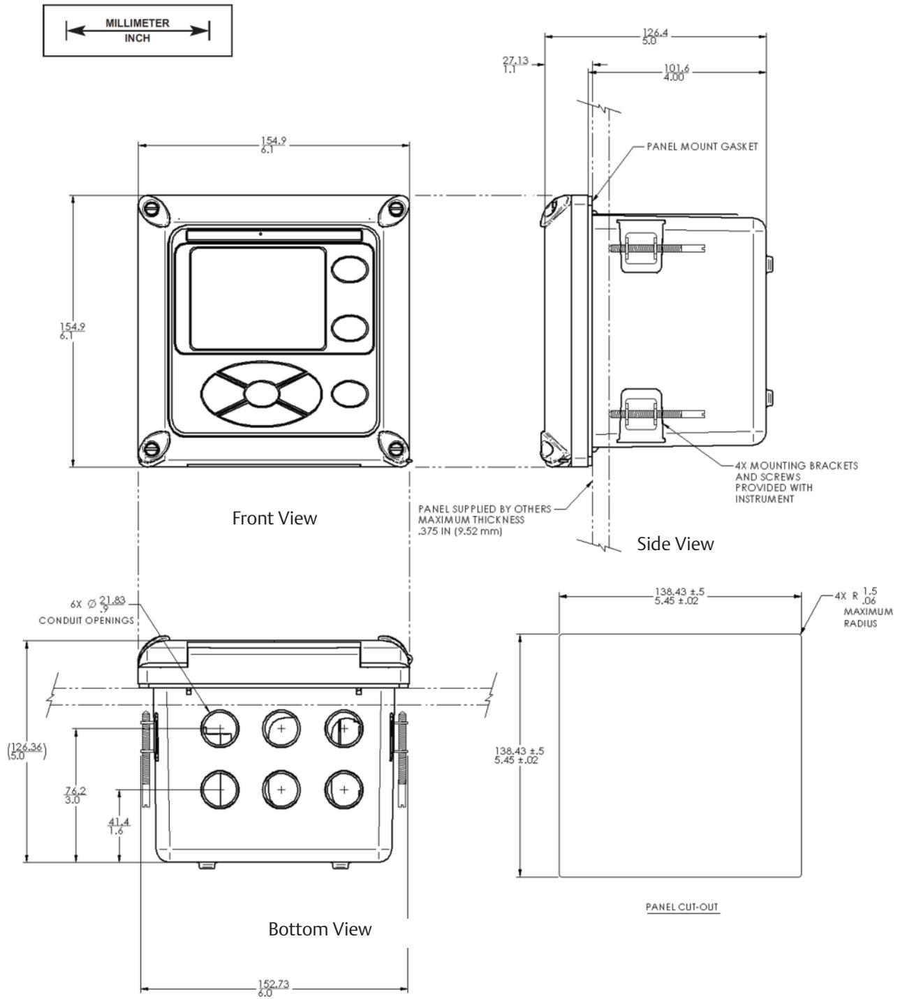
The front panel is hinged at the bottom. The panel swings down for easy access to the wiring locations. Panel mounting seal integrity (4/4X) for outdoor applications is the responsibility of the end user.
