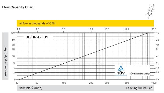
The flow capacity charts have been determined with a calibrated and TÜV certified flow capacity test rig. Volume flow V in (m<sup>3</sup>/h) and CFH refer to the standard reference conditions of air ISO 6358 (20°C, 1bar). Conversion to other densities and temperatures refer to Vol. 1: "Technical Fundamentals".
