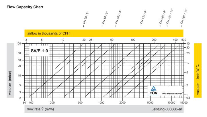
The flow capacity chart has been determined with a calibrated and  $T\ddot{U}V$  certified flow capacity test rig. Volume flow  $\dot{V}$  in (m³/h) and CFH refer to the standard reference conditions of air ISO 6358 (20°C, 1bar). Conversion to other densities and temperatures refer to Vol. 1: "Technical Fundamentals".
