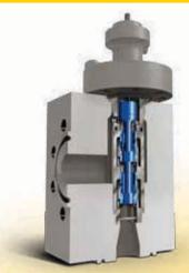
Cavitating Dirty Flow, Customized - Dirty Service Trim (DST) provides cavitation-control for applications with entrained particulate. It uses a combined axial and radial flow path that features large openings allowing particulate up to 19 mm (¾-inch) in diameter to pass through the valve.
