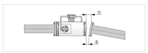
Figure 3-10: Maximum deviation between flanges
