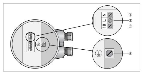
Figure 4-1: Terminals for power supply
