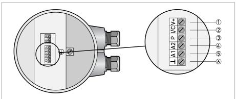
Figure 4-6: Terminals for non Ex HiPower instrument.
