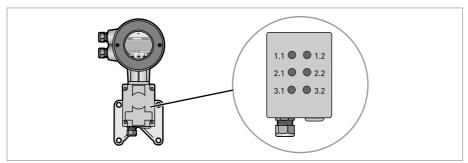
Figure 4-3: Connection of the sensor cables, converter side
