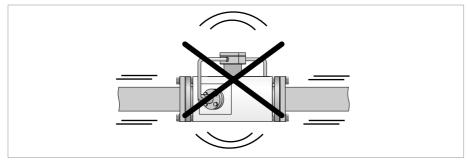
Figure 3-8: Avoid installation in vibrating pipelines.
