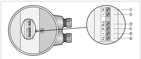
Figure 4-9: Terminals for instrument with Ex-i (Modis)
