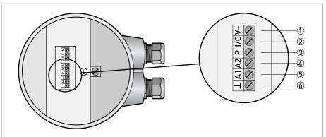
Figure 4-4: Terminals for standard instrument.
