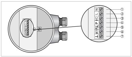
Figure 4-8: Terminals for Ex instrument with NAMUR
