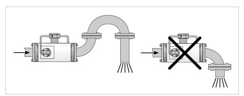
Figure 3-4: Ensure you have a completely filled pipe.
