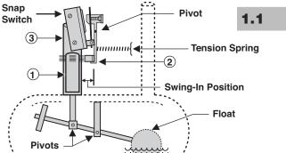
Figure 1 Switch Tripped
