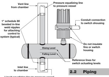
Liquid equalizing line to pressure vessel must be vertical to within three degrees
