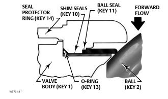
Figure 5. Flow Ring Detail
