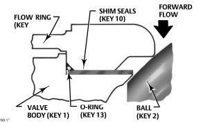
Figure 6. Seal & Backup Ring Assembly
