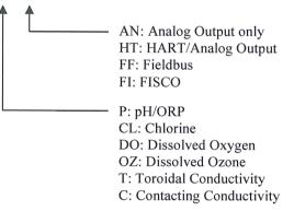
i.e. 1066-P-FF-73 is a Model 1066 intended for measuring pH/ORP with a Fieldbus output.
