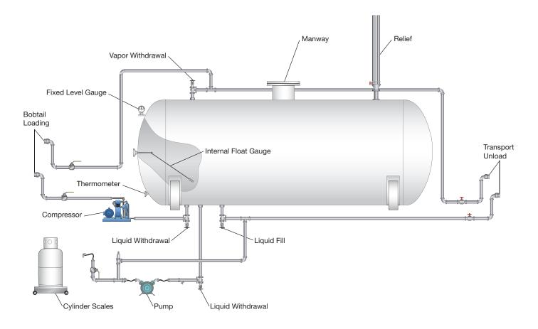
Bulk LPG vessels are used in several types of facilities. They store large amounts of propane to help a supplier meet the demand of the market in the area. Bulk facilities are used to distribute propane to residential and commercial consumers. Vessels are typically designed to load bobtails.
