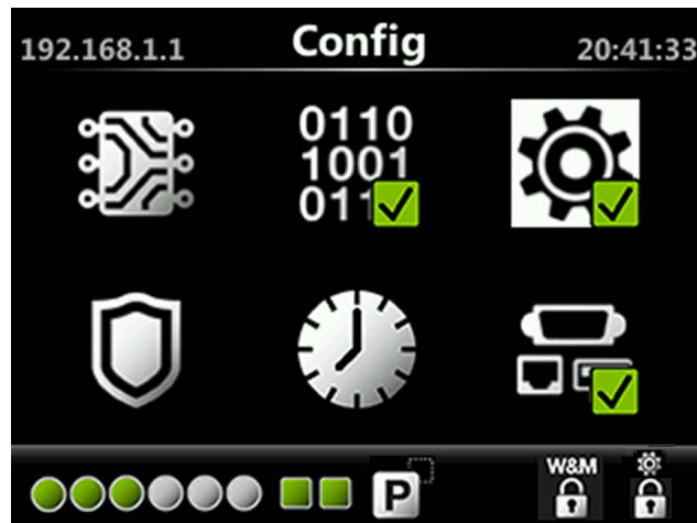
FIGURE 1-8 CIU 888 display: W&M relevant configuration settings are locked
