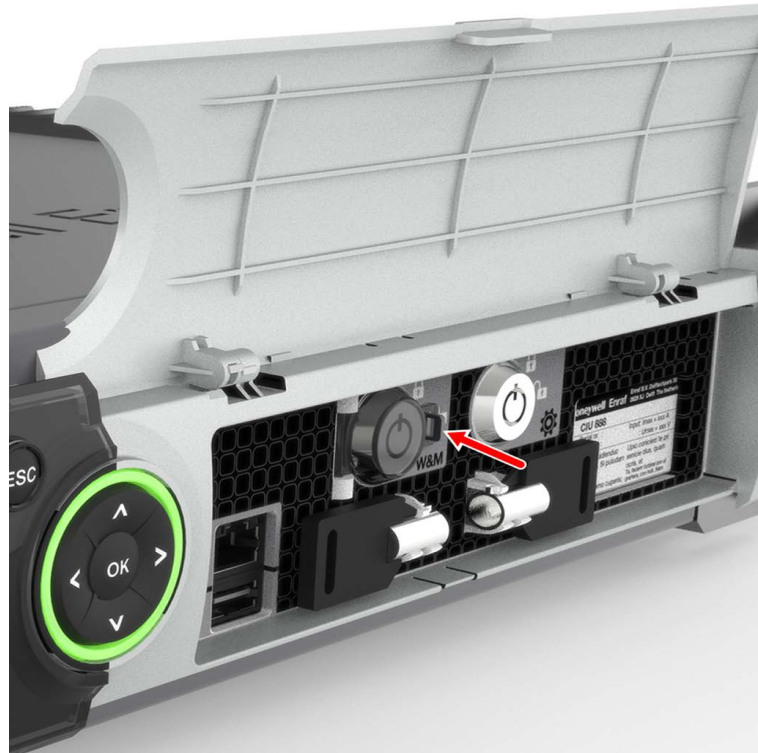
CIU 888: Cover of W&M lock key switch
