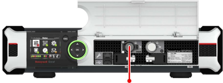
FIGURE 1-7 CIU 888: W&M lock key switch
