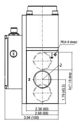
A) Thread M8 - depth 15 (on opposite side); tapped through-hole for M6 screw.
