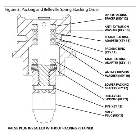
FIGURE 4. Packing and Belleville Spring Stacking Order
