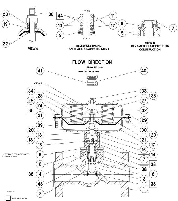
Figure 8. Fisher D3 FloPro Valve Assembly (Spring-to-Open)
