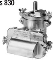
Combination Pressure / Vacuum Relief Vent & Flame Arrester provides pressure and vacuum relief as well as protection from propagation of externally introduced flames. Suitable for NEC Group D (IEC Group IIA) vapors.
