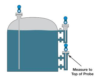
Choosing the proper Guided Wave Radar (GWR) probe is the most important decision in the application process. The probe configuration establishes fundamental performance characteristics. Coaxial, twin element (rod or cable) and single element (rod or cable) are the three basic configurations used today; each with specific strengths and weaknesses.
