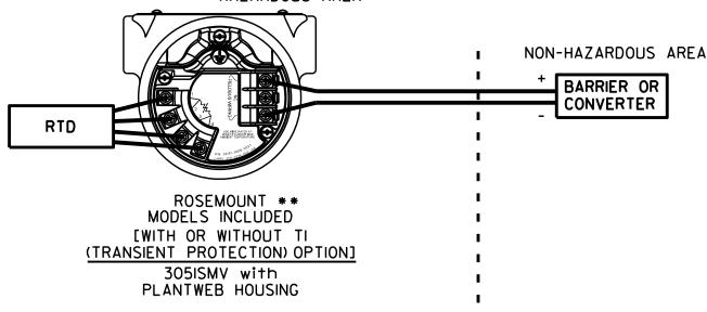
WARNING - EXPLOSION HAZARD - SUBSTITUTION OF COMPONENTS MAY IMPAIR SUITABILITY FOR CLASS I, DIVISION I.
