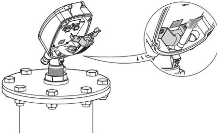
8. Gently connect the antenna cable connector. Make sure the latch is clicked and locking the connector.
