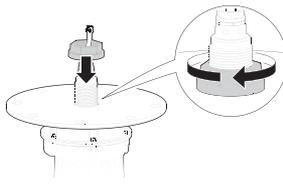
5. Lower the antenna and mounting plate into the fitting location on the silo.
