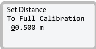
3. Set the distance from the mounting plate (top of the scanner's antenna) to the **Full calibration point/100%** level point.
