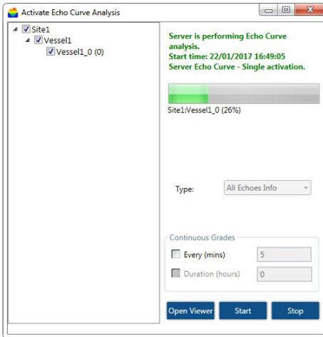
Once the Echo Curve Analysis is complete, the echo curve window will pop up. This function is also available via **Device > Echo Curve Analyze Viewer**.
