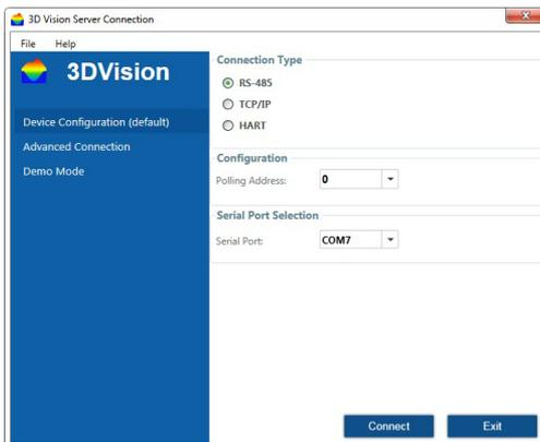
3. Set the correct connection type, polling address, and serial port. Select **Connect**.
