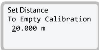
4. Set the distance from the mounting plate (top of the scanner's antenna) to the **Empty calibration point/0%** level point.
