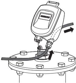
4. Remove approximately 4 in. (100 mm) of the cable mantle and strip approximately 0.4 in. (10 mm) off the edge of each conductor.
