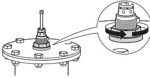
2. Rotate the antenna. **The notch on the top of the thread must be directed toward the center of the silo.**
