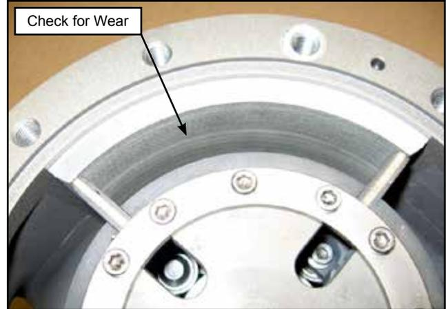
**Figure 29 – Measuring Section Wear**
