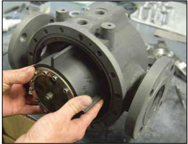
**Figure 38 – Insert Rotor & Blade Assembly into Housing.**
