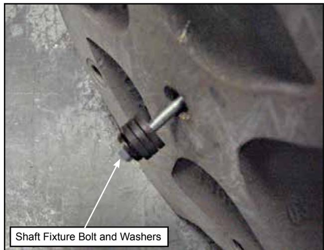
**Figure 39 – Shaft Seating Fixture Bolt and Washers.**
