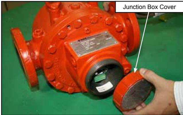
**Figure 3 – Remove Junction Box Cover**
