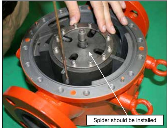
**Figure 14 – Blade to Slot Clearance (Spider Should be Installed)**
