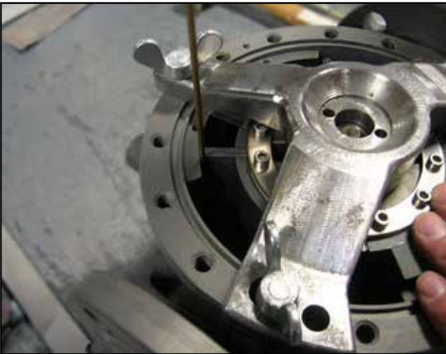
**Figure 41 – Blade Tip to Housing Clearance (at the Measuring Chamber)**
