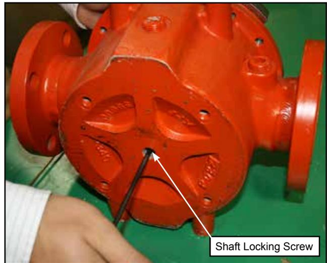
**Figure 19 – Shaft Locking Screw Removal**
