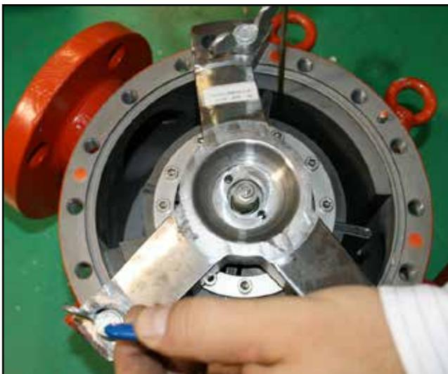
**Figure 17 – Blade Tip to Housing Clearance**
