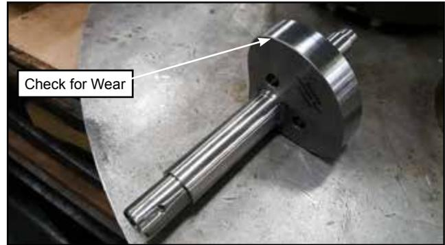
**Figure 26 – Cam and Shaft Wear**
