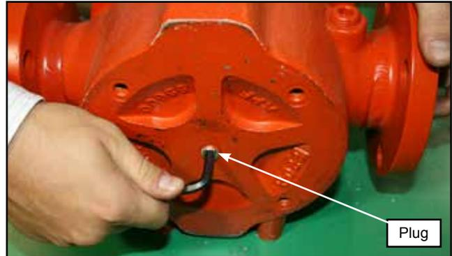
**Figure 18 – NPT Removal**
