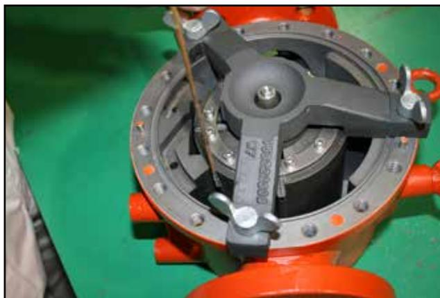
**Figure 11 – Rotor to Block Clearance**
