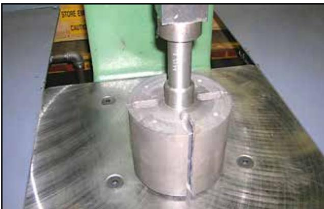
**Figure 25 – Rotor Assembly Bearing installation using Arbor Press**
