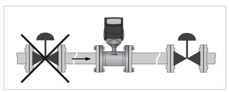
Figure 3-9: Recommended installation: in front of a control valve
