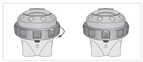
Figure 3-16: Closing of the converter housing
