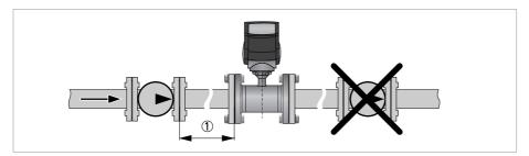
Figure 3-8: Recommended installation: behind a pump
