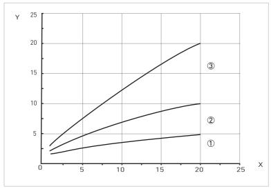
Figure 2-7:  $\mathbf{X}$  = Measuring interval in seconds,  $\mathbf{Y}$  = typical lifetime in years
