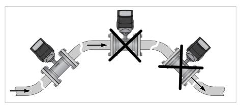
Figure 3-6: Installation in bending pipes
