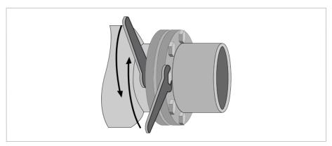
Figure 3-14: Tightening of bolts
