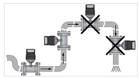
Figure 3-5: Installation in bending pipes
