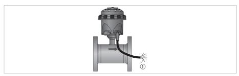
Figure 4-7: Output cable at IP68 compact version
