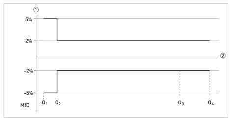
Figure 2-2: ISO flow rates added to figure as comparison towards MID  $\mathbf{X}$ : Flow rate
