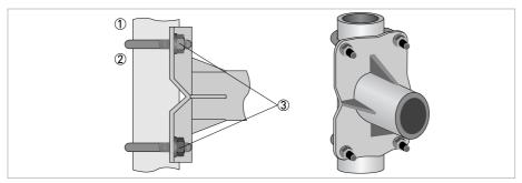
Figure 3-15: Pipe mounting of the field housing
