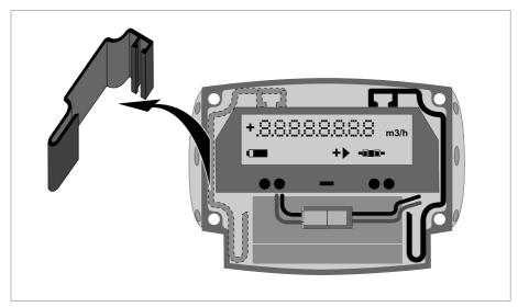
Figure 4-5: Removing side cap
