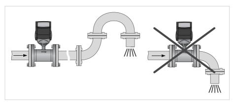
Figure 3-7: Installation in front of an open discharge
