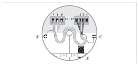
Figure 4-3: Cable connection at sensor side, standard cable
