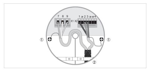
Figure 4-4: Cable connection at converter side, standard cable
