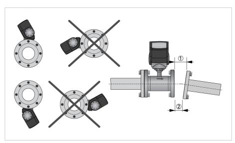
Figure 3-12: Mounting position and flange deviation
