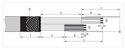
Figure 4-2: Preparation of standard cable on sensor side
