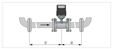
Figure 3-3: Minimal inlet and outlet
