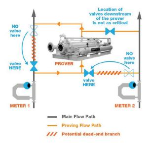
Sufficient back pressure must be maintained on both the prover and the meter to avoid vapor breakout and to maintain a stable flow rate during displacer launch and travel. Minimum recommended back pressure is shown by Equation 4 (from API MPMS Ch. 5.6).
