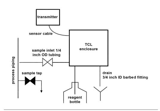
Figure 3-1: Installing the Sample Conditioning Enclosure
