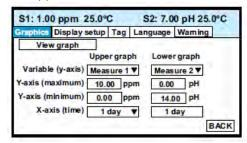
2. Configure the displayed variable, the maximum and minimum values for the Y-axis, and the time scale.
