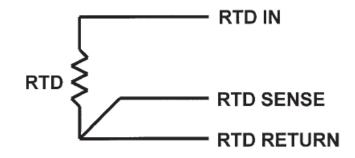
Although only two wires are required to connect the RTD to the transmitter, using a third (and sometimes fourth) wire allows the transmitter to correct for the resistance of the lead wires and for changes in the lead wire resistance with temperature.
