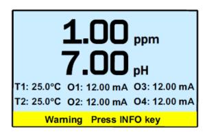
The following abbreviations are used in the lower two lines of the display. The number following the display refers to the sensor, alarm relay, or output.
