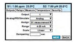
13. To view the next screen, use the navigation keys (either **Down** or **Right**) to move the cursor to **NEXT** and press **ENTER/MENU**.
