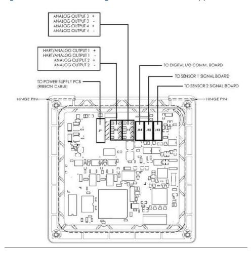
Figure 12-1: Main Board Showing Connections to Sensor Board(s)
