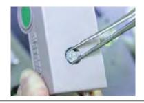
8. Slide the pump assembly out of the air pump body.
