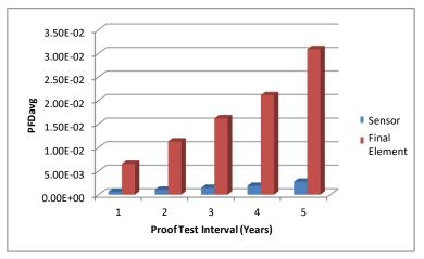
Figure 3: PFD<sub>avg</sub> versus Proof Test Interval
