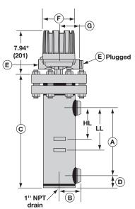
Flanged Top Chamber w/NPT or Socket weld Side/Side Connections (H15, H32, H52)
