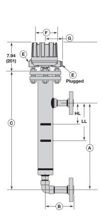
Flanged Top Chamber Side/Side Flange Connections (C74 only)
