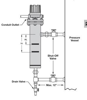
Figure 3 Typical Piping Arrangement
