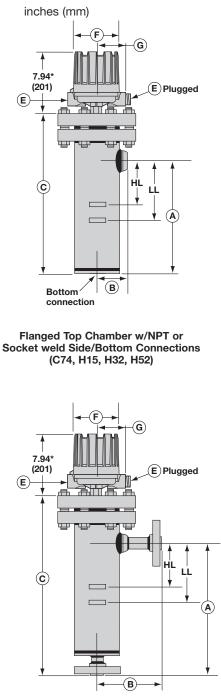
Flanged Top Chamber Side/Bottom Flange Connections (C74, H15, H32, H52)
