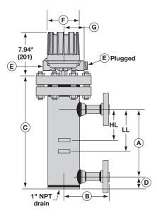
**Flanged Top Chamber** Side/Side Flange Connections (H15, H32, H52)
