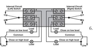
Figure 6 Terminal Connections DPDT Switch Mechanism Series HS
