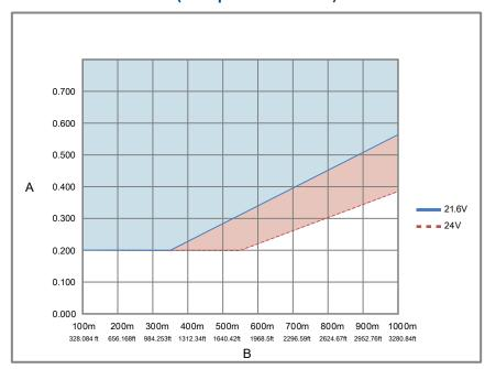
Figure 1-2: Minimum wire area (mm<sup>2</sup> per meter or foot)
