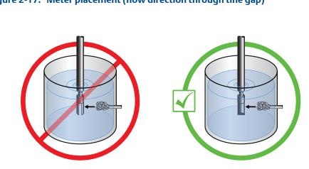
Figure 2-17: Meter placement (flow direction through tine gap)
