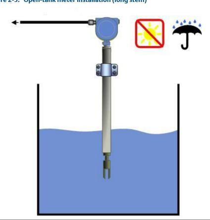
Figure 2-5: Open-tank meter installation (long stem)
