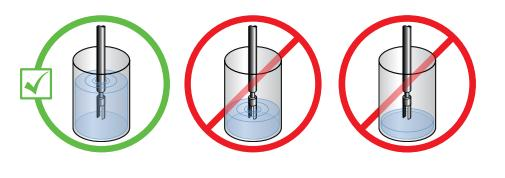
5. Confirm the meter placement has allowed for the flexing of the tank lid to prevent the meter from being pushed towards a tank wall or into the path of disturbed flow.
