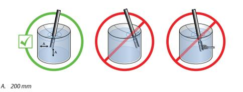
6. Confirm the meter tines are placed away from objects and disturbed flow.
