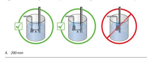
Figure 2-8: Meter placement (distance from objects and disturbed flow)
