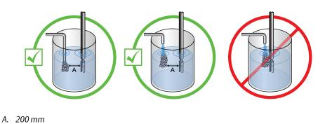
7. If flow exists, confirm the meter tines are aligned so that the flow is directed towards or through the gap between the tines.
