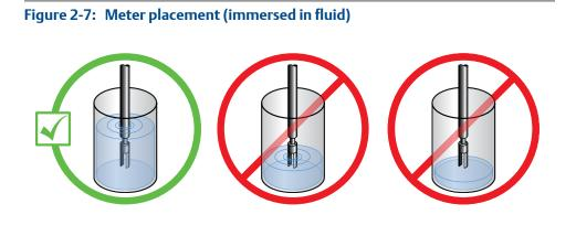
4. Confirm the meter tines are placed away from objects and disturbed flow.
