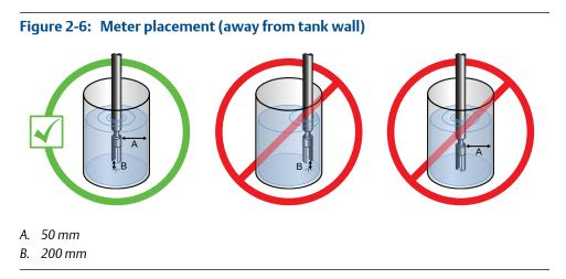
3. Confirm the meter tines are immersed in fluid.
