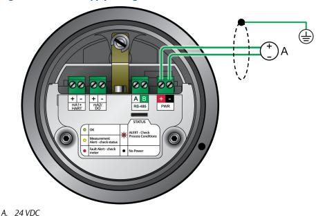
Figure 1-4: Power supply wiring terminals
