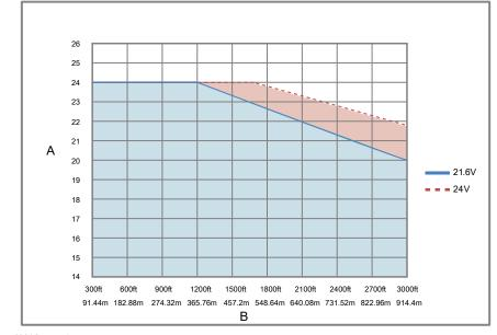
Figure 1-1: Minimum wire gauge (AWG per foot or meter)
