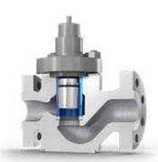
Multiple passages break up the large turbulent stream into many small, independent jets to quiet noise
