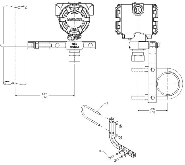
A. 2-in. U-bolt for pipe mounting (clamp shown) B.  $^1/4x\ 1^1/4$  bolts for transmitter mounting
