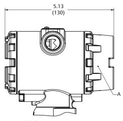
A. Digital display cover B. 2 x ½–14 NPT conduit connection
