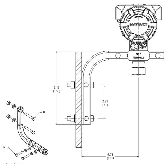
A.  $^1/4 \times 1^1/4$  bolts for transmitter mounting B.  $^5/16 \times 1^1/2$  bolts for panel mounting (not supplied)
