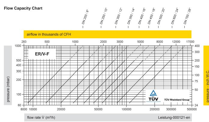
The flow capacity chart has been determined with a calibrated and TÜV certified flow capacity test rig. Volume flow  $\dot{V}$  in (m³/h) and CFH refer to the standard reference conditions of air ISO 6358 (20°C, 1bar). Conversion to other densities and temperatures refer to Vol. 1: "Technical Fundamentals".
