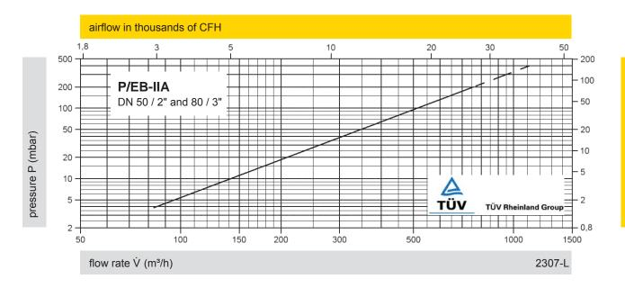
The flow capacity charts have been determined with a calibrated and TÜV certified flow capacity test rig. Volume flow  $\dot{V}$  in (m³/h) and CFH refer to the standard reference conditions of air ISO 6358 (20°C, 1bar). Conversion to other densities and temperatures refer to Vol. 1: "Technical Fundamentals".
