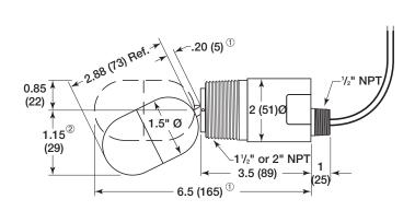
TK1 with threaded connection and SPST or SPDT switch with flying leads
