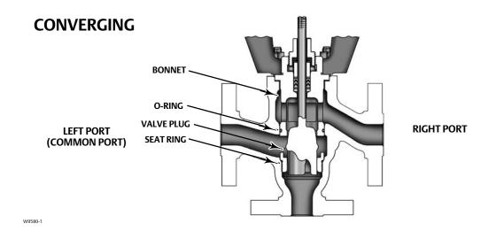
Figure 7. Fisher GX 3-Way Flow Directions for Side Port Common Converging Constructions
