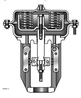
The GX 3-Way uses a multi-spring, pneumatic diaphragm actuator (see figure 15). It is capable of air supply pressures up to 5.0 barg (72 psig), allowing valve shutoff at high pressure drops (see table 8).
