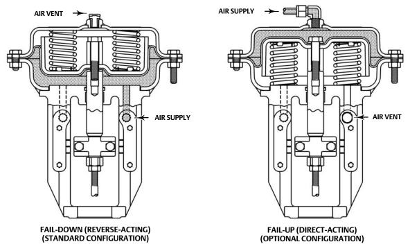
Integrated Air Supply. When mounted with the DVC2000 digital valve controller, the GX 3-Way uses an integrated actuator air supply system. In the fail-down configuration, air is supplied to the lower
