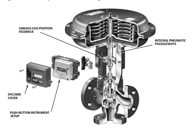
Optimized valve and actuator system. Product simplicity and ease of selection form the foundation of the GX 3-Way. Mounted with a digital or analog positioner, the GX 3-Way provides high performance control across a wide range of process applications.
