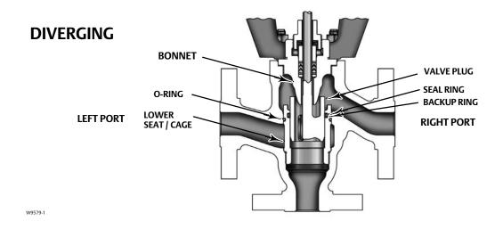
Figure 9. Fisher GX 3-Way Flow Directions for Bottom Port Common Diverging Constructions
