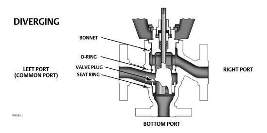
Figure 5. Fisher GX 3-Way Flow Directions for Side Port Common Diverging Constructions
