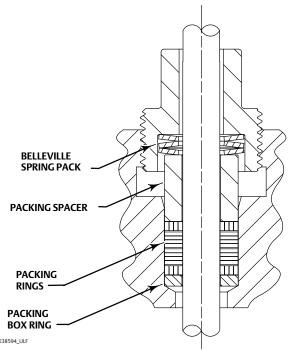
STANDARD BONNET WITH OPTIONAL ENVIRO-SEAL LIVE-LOADED GRAPHITE ULF PACKING SET (STANDARD ON HIGH TEMPERATURE CONSTRUCTION)
