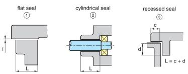
The dimensions given depend on the seal and volume of the enclosure and gas groups. Example: with a seal length L=12.5~mm and an enclosure volume  $\leq 100~\text{cm}^3$ , the MESG "i" will be:
