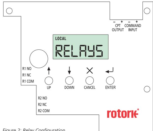
Figure 2: Relay Configuration
