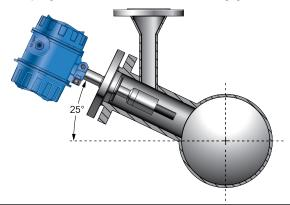
Insert a purge/drain connection on the upper part of the T-piece. You can use the purge connection to flush the pipe if necessary.
