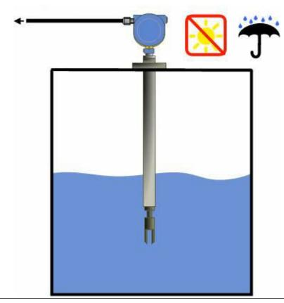
2. To vary the insertion depth of the meter, mount the meter on a standoff section that attaches to the flange (not provided).
