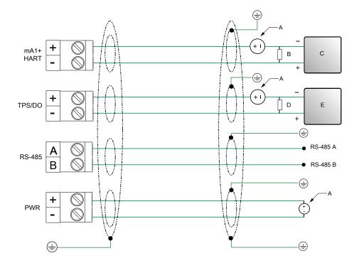
Figure 4-1: Wiring the TPS or Discrete Output version
