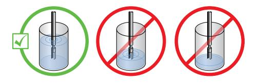
4. Confirm the meter tines are placed away from objects and disturbed flow.
