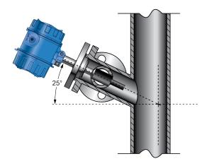
Insert a purge/drain connection on the side of the T-piece. You can use the purge connection to flush the pipe if necessary.
