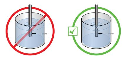
6. Confirm the meter tines are kept away from deposit buildup.
