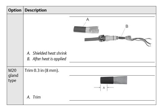
8. Assemble the gland by folding the shield or braid back over the clamping insert and 0.125 in (3 mm) past the O-ring.
