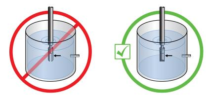
8. Confirm the meter tines are kept away from deposit buildup.
