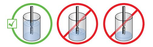
5. Confirm the meter placement has allowed for the flexing of the tank lid to prevent the meter from being pushed towards a tank wall or into the path of disturbed flow.
