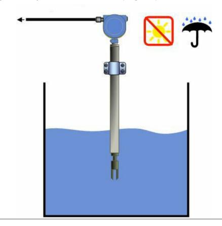
2. Confirm the meter tines are away from the tank wall.
