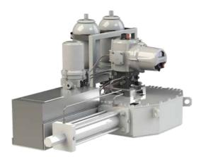
The Skilmatic SI4 quarter-turn actuators offer the flexibility of customisation to suit specific applications and process conditions. The high pressure actuators are self-contained and can operate either a spring-return or double-acting scotch yoke drive. This eliminates the high installation and maintenance costs associated with conventional electrohydraulic systems which utilise central hydraulic power units.
