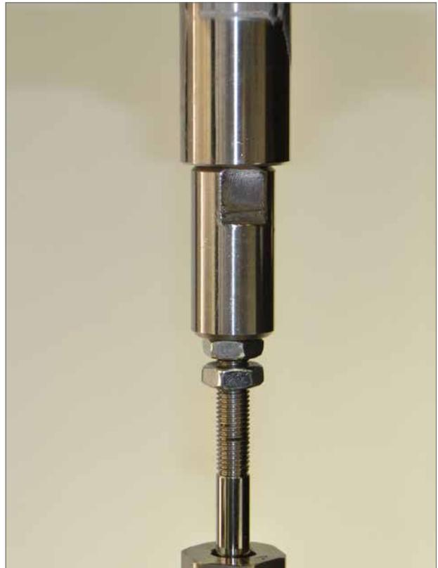
Fig 6.7 Connection of valve shaft and actuator shaft
