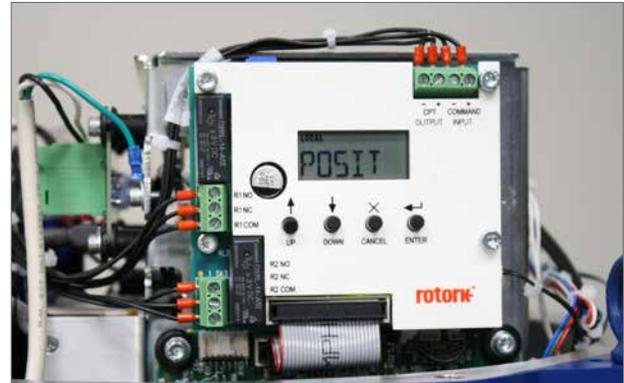
Fig 7.32 Control input connection
