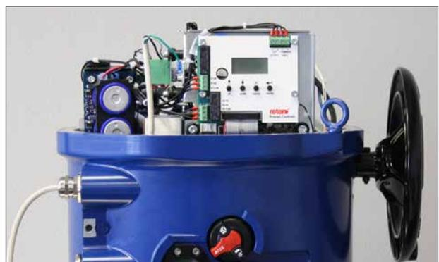
Fig 6.14 Internal electronics
