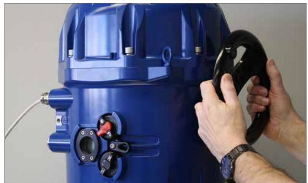
Fig 6.3 Manual operation of the actuator
