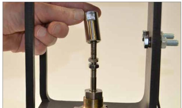
Fig 6.4 Coupling attachment to valve shaft
