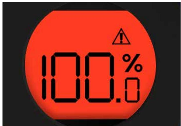
Fig 5.3 Actuator flashes Red and White alternately when power failure occurs
