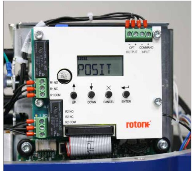
Fig 5.4 Internal interface
