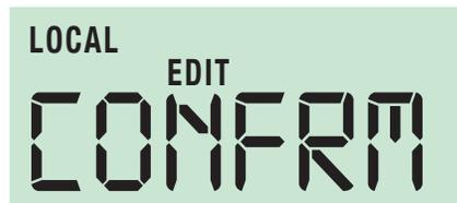
Fig 10.2 Confirm setting overwrite
