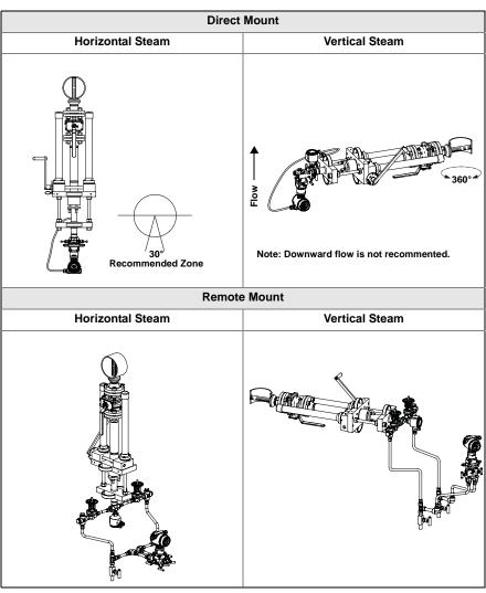
Figure 2-12. Top Mounting for Steam
