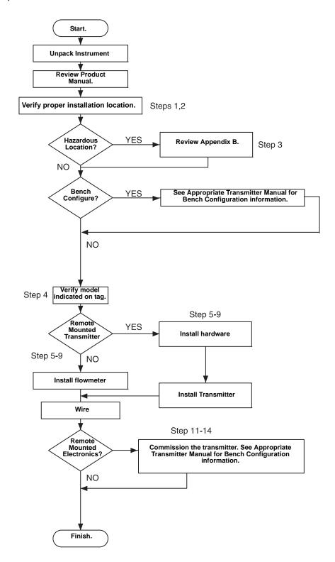
The following list is a summary of the steps required to complete a flowmeter installation. If this is a new installation, begin with step 1. If the mounting is already in place, verify that the hole size and the fittings match the recommended specifications (see Table 2-3 on page 2-19) and begin with step 5.
