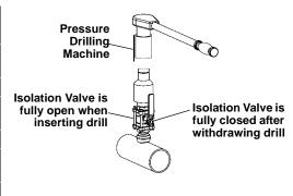
Step 5: Remove the Drilling Machine
