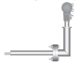
**BYPASS PACKAGE:** The Bypass Oxygen Analyzer Package consists of a 1 inch Inconel tube; a 2 inch Inconel tube; a Hagan industrial quality oxygen analyzer and an external stainless steel housing. Mounting angles of the external analyzer can vary according to application requirements.
