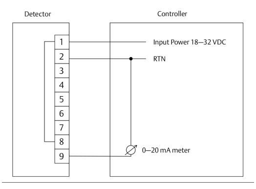
Figure B-4: 0-20 mA Output Configuration 1A (Converted to Source 3-Wire)
