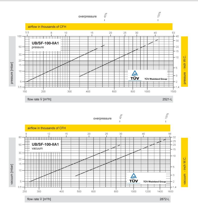
The flow capacity charts have been determined with a calibrated and TÜV certified flow capacity test rig. Volume flow  $\dot{V}$  in [m<sup>3</sup>/h] and SCFH refer to the standard reference conditions of air ISO 6358 (20°C, 1bar). Conversion to other densities and temperatures refer to Technical Fundamentals.
