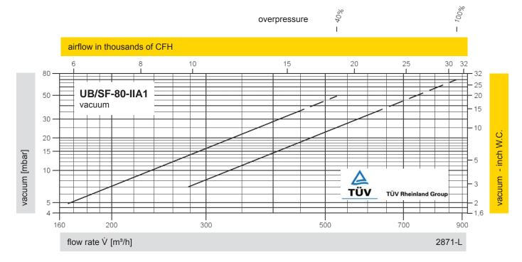
The flow capacity charts have been determined with a calibrated and TÜV certified flow capacity test rig. Volume flow  $\dot{V}$  in [m<sup>3</sup>/h] and SCFH refer to the standard reference conditions of air ISO 6358 (20°C, 1bar). Conversion to other densities and temperatures refer to Technical Fundamentals.
