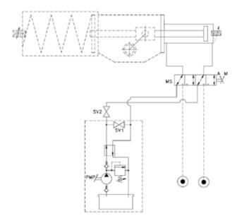
Figure 18 – Hydraulic Diagram of Manual Override for LHS Single Acting
