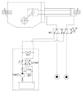
Figure 20 – Hydraulic Diagram of Manual Override for LHS Double Acting
