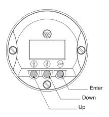
The Eclipse transmitter comes partially configured from the factory but can be reconfigured in the shop (disregard fault message due to unattached probe). The minimum configuration instructions required in the field follow. Use the information from the operating parameters table in Section 2.1.2 before beginning configuration.
