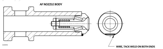
17. Reassemble in the following order: nozzle sleeve gasket (key 47), nozzle body flange gasket (key 48), spray nozzle/sleeve assembly (key 30 and 37), nozzle body flange (key 20), washers (key 59), and stud nuts (key 58). It is required to replace the nozzle sleeve gasket (key 47) and nozzle body flange gasket (key 48) with new gaskets each time the nozzle body flange (key 20) is removed.
