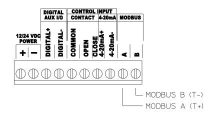
Figure 8. Wiring - Auxiliary Digital I/O set to input (40080=0)
