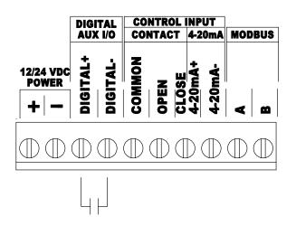
Figure 9. Wiring - Auxiliary Digital I/O set to output (40080=1)
