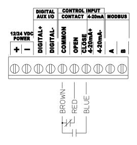
Figure 6. Wiring - Single Dry Contact
