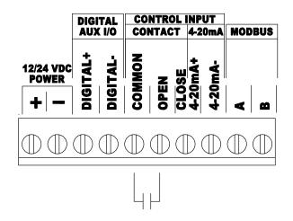
Figure 7. Wiring - Modbus Input
