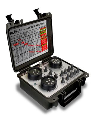
**The NEW Scully Rack Tester** is an advanced, comprehensive, portable tester approved for testing in hazardous locations. It allows Scully customers and field personnel to quickly assess any Scully overfill prevention, grounding and vehicle identification rack controller for proper equipment operation. In the event of a malfunction, it facilitates problem isolation and resolution.
